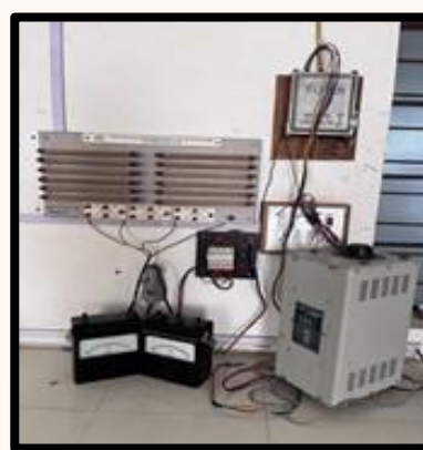
3 Phase Star/Delta Measurement
