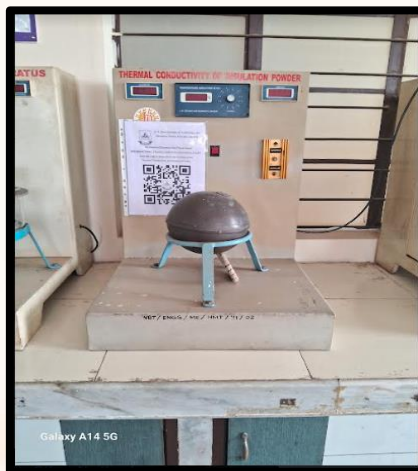
Thermal conductivity of insulation powder
