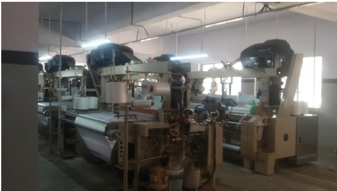
Figure shows the water jet machine for making cloth material
